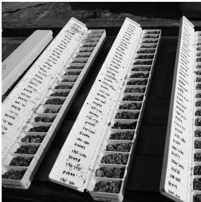
**Pictured:** Drilling chip samples MB Project, Nevada
